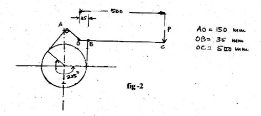
the necessary force (P) for the clockwise and anticlockwise rotation of the drum, and (ii) the value of 'OA' for the brake to be self-locking, when the drum rotates clockwise.
